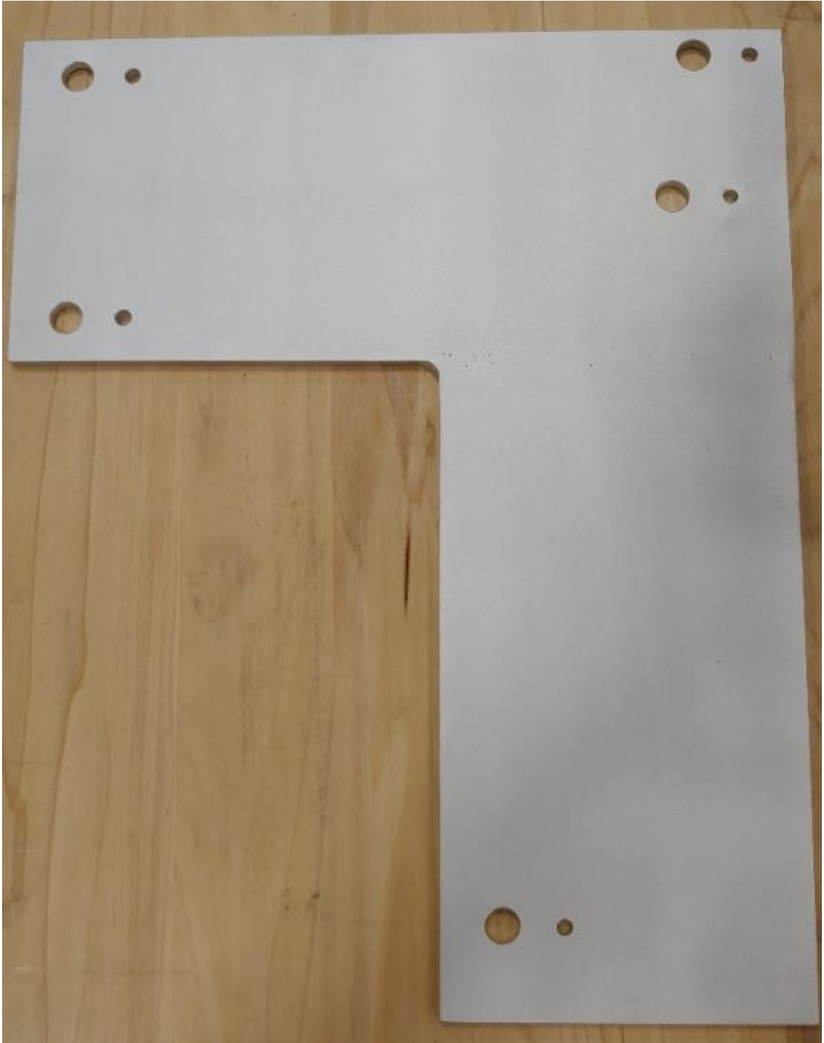
FIGURE C-2 VW CRACK METER INSTALLATION TEMPLATE
